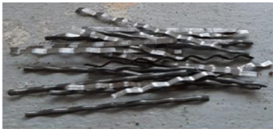
Fig.1 Flat crimped steel fibres
